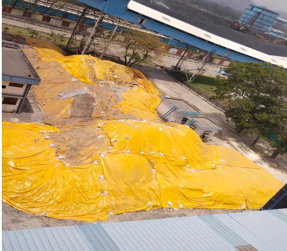
FIGURE 8& 9: FGD GYPSUM STORED OUTSIDE SHED, COVERED WITH IMPERVIOUS SHEETS
