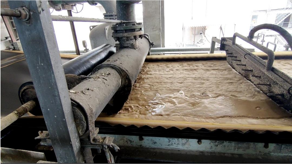
FIGURE 4: VACUUM FILTER BED
