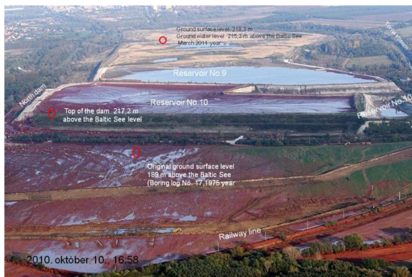
Picture and altitude figures of the reservoir system after the embankment failure in October 2010 ( http://redsludge.bm.hu )
