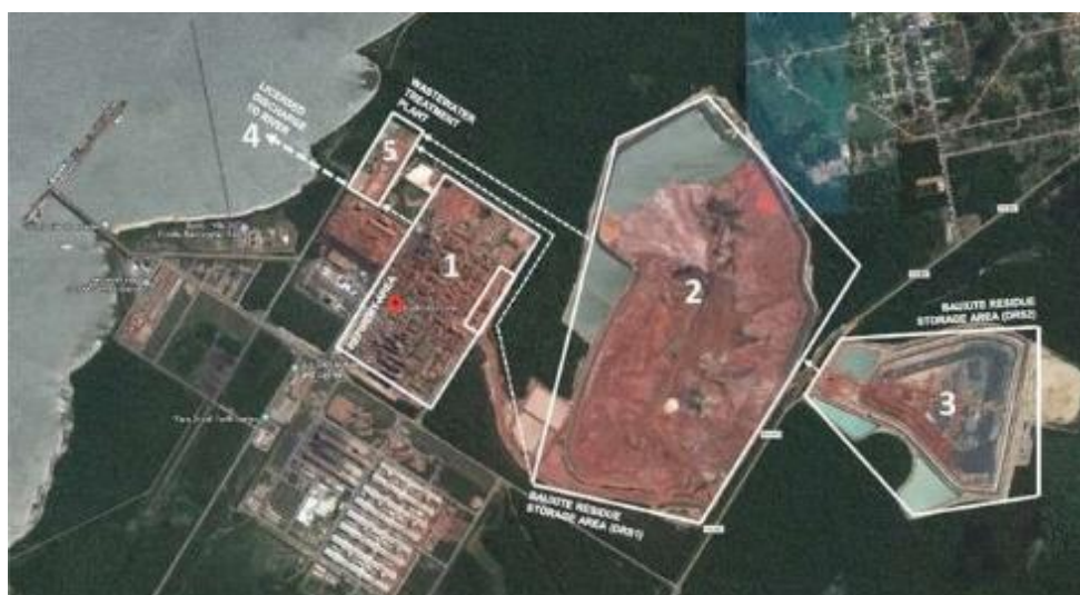
Figure 23: Satellite view of Alunorte and the Pará River with illustration of production and associated facilities (1. Refinery area; 2. Bauxite Residue Storage Area DRS1; 3. Bauxite Residue Storage Area DRS2; 4. Licensed discharge to Pará River; 5. Wastewater treatment plant)
